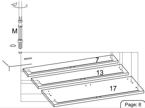
Take the drawer front A (7), drawer front B (13) and drawer front C (17). Screw the twelve connecting bolts (M) into the drawer fronts. Tighten
