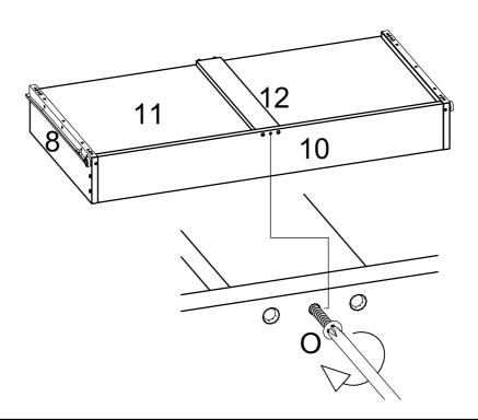
Take the drawer front A (7). Put a few drops of glue (N) into the two holes.
