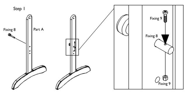
Insert the stop peg (fixing 8) through the outside of the stop peg crib foot (part A) and fix using the stop peg nut and bolt (fixing 9) as shown. Tighten all fixings fully.
