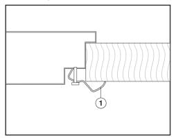
■ Secure the hob using the brackets ① supplied.
