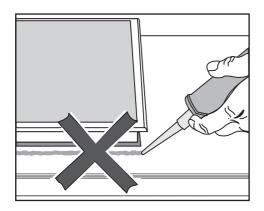
Do not use sealant between the hob and the worktop. This could result in damage to the hob or the worktop if the hob ever needs to be removed for servicing.
