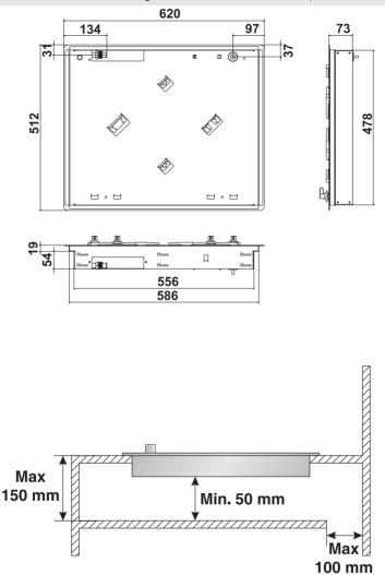
IMPORTANT: if the appliance is mounted on a unit, make sure that a separating shelf is installed, as shown in the figure.
