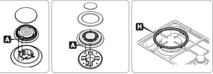
The burner controlled by each knob is shown next to the knob. The appliance is equipped with an electrical ignition device. Simply press the knob and turn it anti-clockwise to the maximum flame symbol  $\bigwedge$ , until the burner lights.
