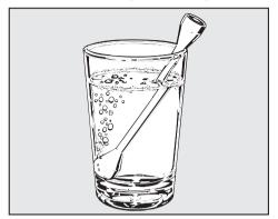
When reheating liquids, always place the boiling rod supplied into the cup or glass.
