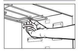
■ To lower the top heat/grill element, the nut needs to be unscrewed.
