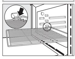
To remove the rack, lift it upwards slightly at the front when the safety notches connect with the sides of the oven.
