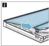
Push down on the intermediate panel around a, carefully lift the holder b until it can be pulled out (Fig. 3).
