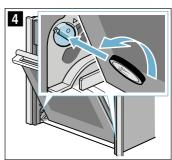
Left-hand lock: Anti-clockwise Right-hand lock: Clockwise
