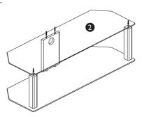
5. Place short legs onto panel and screw barrel nuts onto all threaded bars.
