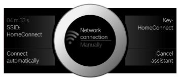
Use the SSID "HomeConnect" and the key "HomeConnect" to register the mobile device on the oven network.
