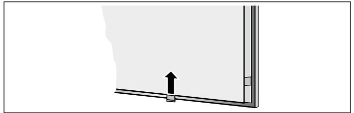
4. Take the metal grease filter out of the holder.
