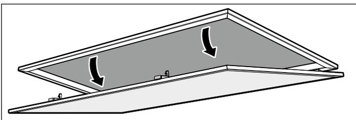
3. Press the lock on the metal grease filters.
