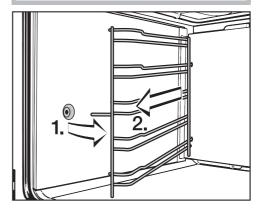
■ Pull the side runners out of holder (1) at the front of the oven and then pull them out of the oven (2).
