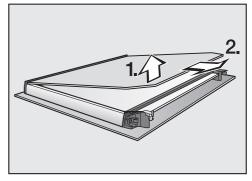
■ Carefully lift the inner pane up and out of the plastic strip.
