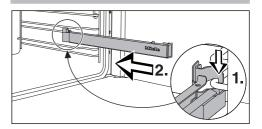
■ Hook the FlexiClip runner onto the front of the lower rail of a side runner (1.) and then push it along the rail into the oven compartment (2.).
