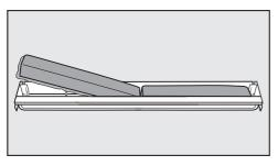
■ Remove both charcoal filters and place the new filters with the framed edge pointing downwards in the holder.
