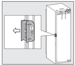
■ Open the appliance door and remove the red safety catch ① (depending on model).
