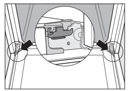
The door is connected to each door hinge by retainers.
