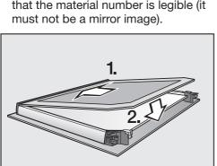
■ Push the inner pane with the matt printed side facing downwards into the plastic strip and place it between the retainers.
