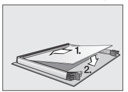
■ Refit the middle pane in such a way that the material number is legible (it must not be a mirror image).
