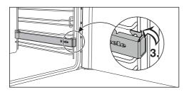
■ Then secure the FlexiClip runner to the lower of the two rails as illustrated (3).
