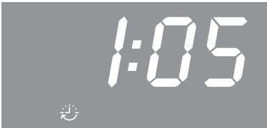
The cooking duration is saved and then counts down in minutes, with the last minute counting down in seconds.
