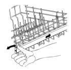
**Version B:** with adjustment in **three positions** on both sides. The sides of the basket **must always be set at the same height**.
