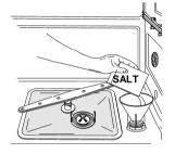
When using water of medium hardness, the regenerating salt container should be refilled after approximately **20 washing cycles**. The salt container can hold approximately **1.7 Kg** of salt in grains. The container is situated at the bottom of the dishwasher. After removing the lower basket, unscrew the salt container cap by turning it anticlockwise and pour in the salt using the funnel supplied with the dishwasher. Before replacing the cap, remove any salt residues from around the opening.
