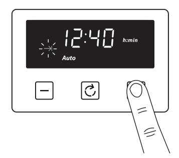
The auto cooking symbol disappears from the display once the time, the required cooking settings and temperature have been set. The appliance will not be switched on until the set cooking start time, that is the difference between the cooking end time and the cooking duration.
