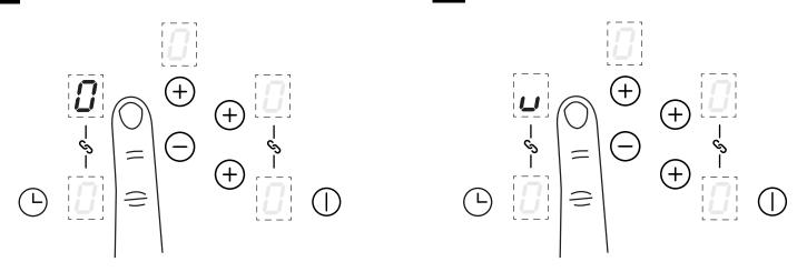
The "u" symbol can be found between power level "0" and "1". Use the relevant cook zone plus key and central minus key to scroll through the power levels.
