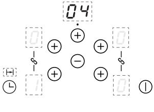
When the time is up, the timer display will flash, beep and the cook zone will automatically switch off. Touch any key to stop the beeping.
