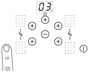
The time will set when no key is pressed after 1 second. A dot will flash in the timer display. The time will count down
