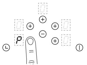
For quick operation, touch the minus key for quicker access to the Power Boost level.
