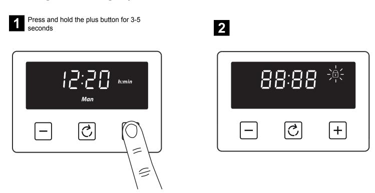
Once the Key lock is active, the buttons will be inactive. A two beep signal will be heard if the buttons are pressed.
