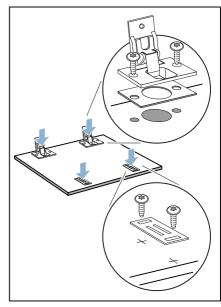
**10.** Put the hinges in the appliance (1 + 2), push on the cover panels (3) and screw them in place (4).
