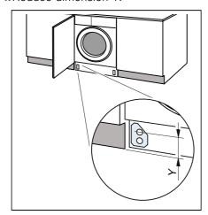
**15.** Screw the spacers in as per the dimensions.
