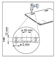
9. Put the hinges in the holes and screw them in. Screw in the counter plates for the magnetic catches.
