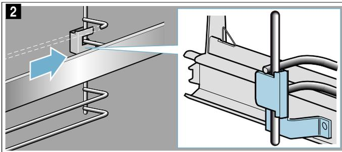
3. Push on the "PUSH" tab and swing the rail in so that the retainer ends up between the two bars (fig. 3).
