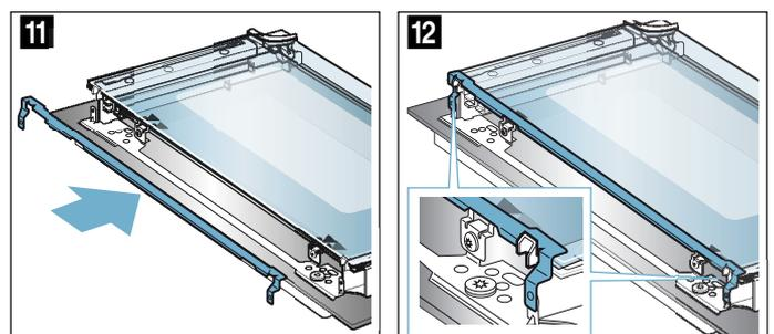
12. Attach the cover and use two screws to secure it (fig. 13).
