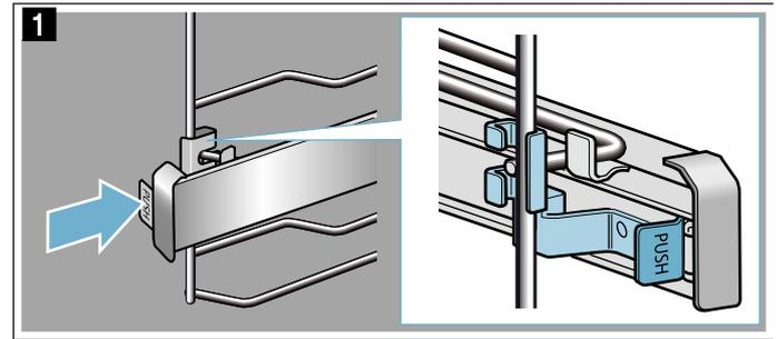
2. Keep the "PUSH" tab pushed back and swing the rail out (fig. **2**).
