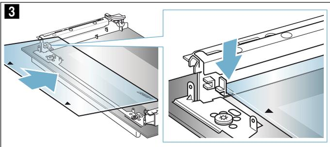
4. Slide the other inner panel back in and make sure that the number on the inner panel is to the bottom right (fig. **4**).
