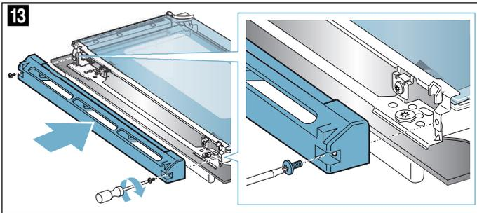
13. When fitting the appliance door, ensure that both hinges are inserted straight into the opening (fig. 14). Place both hinges at the bottom on the outer panel and use them as a guide. Ensure that the hinges are inserted into the correct opening. You must be able to insert them easily and without resistance. If you can feel any resistance, check that the hinges are inserted into the correct opening.
