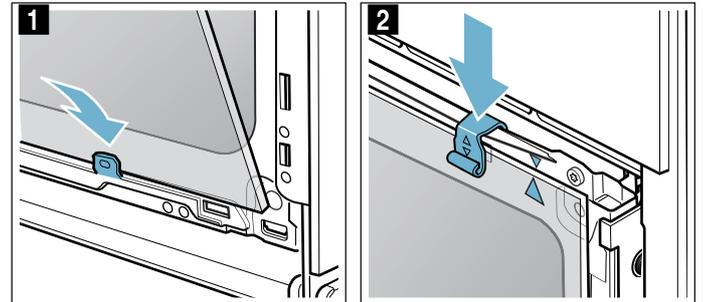
3. Insert the front panel at the bottom into the retainers (figure 3).
