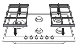
2. Lay the centre grid engaging the notches in the teeth of the lateral grids.
