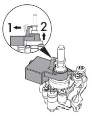
Use a 7-mm spanner to remove the nozzle and replace it with the new one for the required gas supply, following the indications given in the relevant tables (see Gas types and Countries").
