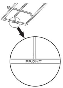
• Position the grids so that the marks "**FRONT**" are facing the hob knobs.
