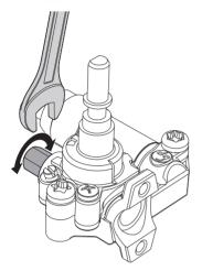
The nozzle tightening torque must be no more than 3 Nm.
