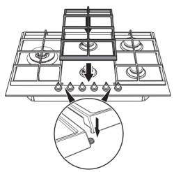
In addition, pay attention to the mark "**FRONT**" under each grid at the front, as a further help to correctly position the grids on the hob.
