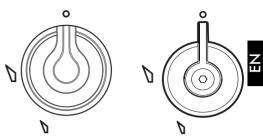
Used for lighting and adjusting the hob burners. Press and turn the knobs anticlockwise to h in order to light the relative burners. Turn the knobs to the zone between the maximum h and minimum hsetting to adjust the flame. Return the knobs to the position O to turn off the burners.
