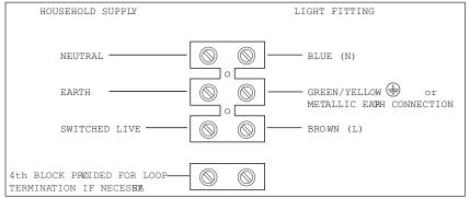
A fourth connection block is provided should you need it to make a loop connection. You must then wrap the connection block in tape covering at least 2cm of the wiring on each side
