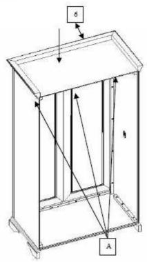
Place the top (6) and attach with screws (A) to side panels(3) and front frame, again through batons.
