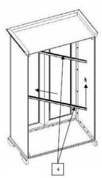
Insert the hanging rails(4) in the support brackets.
