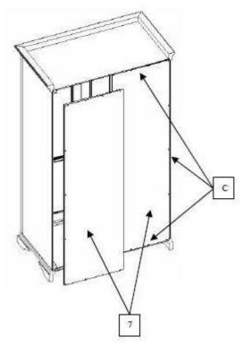
Insert the back panels(7) as shown and attach with screws(C) provided
