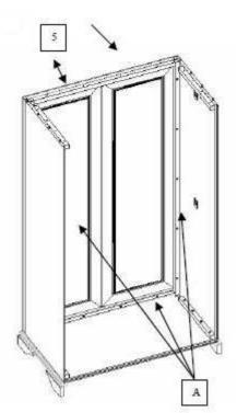
Place the front frame with two doors (5) and attach to side walls and bottom panel/base with screws (A) thought the batons.
