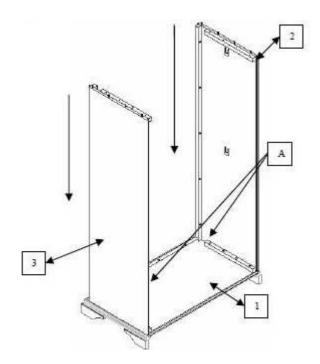
Place the LH side panel (2) onto the bottom panel, ensuring it is properly secured in existing holes in the base, then attach with screws (A) trough batons. Repeat step for RH side panel (3) .
