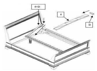
Push the plastic sockets (D) onto each end of the slats slotting one end into the centre rail cap (fitted) and pushing down the other end to secure in place using holes provided.
