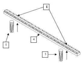
Attach centre support rail feet (5) using wood screws (E) under the central support rail (4)
