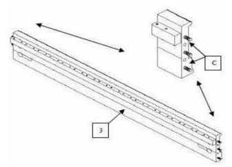
Insert wooden dowels (C) in the holes provided at both ends of the side rails (3)
