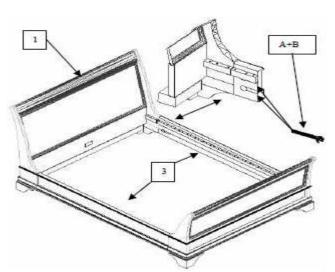
Place cam (B) over the bolt (A) and insert them in holes provided, on the inside of the siderail (3) and then tighten using a screwdriver
