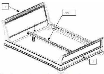
Push the central support rail (4+5) in place as arrows show to engage with clips on the head board (1) and foot board (2)
