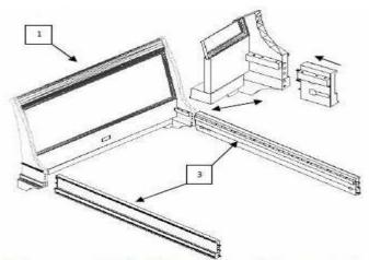
While one person holds head board (1) upright the other person slides the rails (3) over the wooden dowels and flush with the head end.
