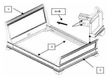
Both people hold the foot board (2) and LIFTING TOGETHER slot the side rails (3) over the wooden dowel (C) and repeat as in step 3
