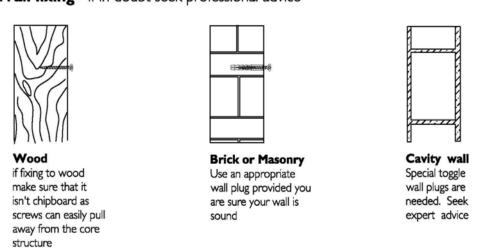
7. Attach the wall bracket using screws suitable for your type of wall, see wall fixing above.
