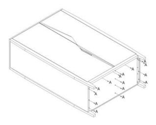
4. Attach the Top panel 5 onto the side panels and middle panel using the 30mm screws.
