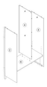
3. Attach the door frame I onto the side panels 2,3 and middle panel 4, using 30mm screw A. Then fix the bottom 6 onto the side panels , middle panel and door frame, using the 30mm screw A.
