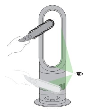
Ensure the heater is unplugged and has been allowed to cool. Look for blockages in the air inlet holes and in the small aperture inside the air loop amplifier. Use a soft brush to remove debris.
