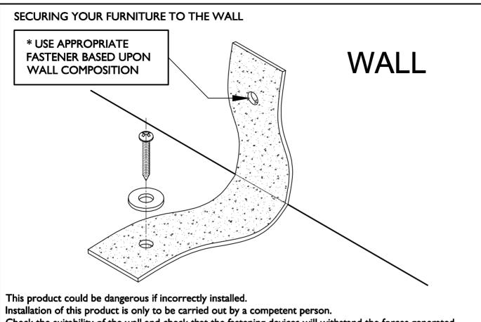
Check the suitability of the wall and check that the fastening devices will withstand the forces generated.
