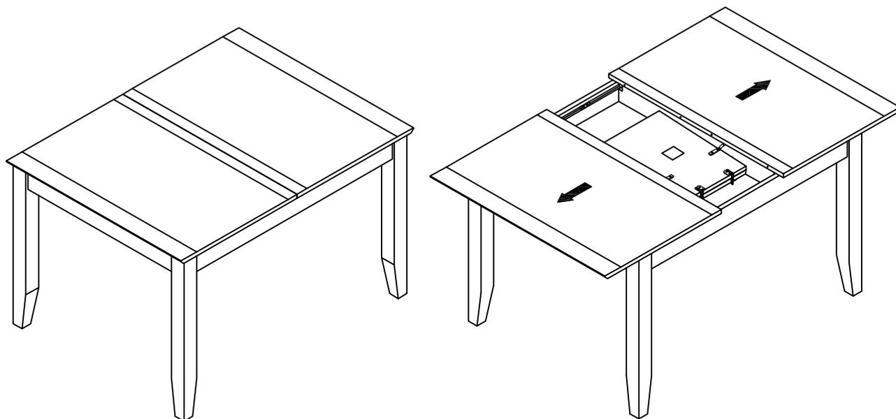
**Step 4** : Rotate the extension leaf out as shown.
