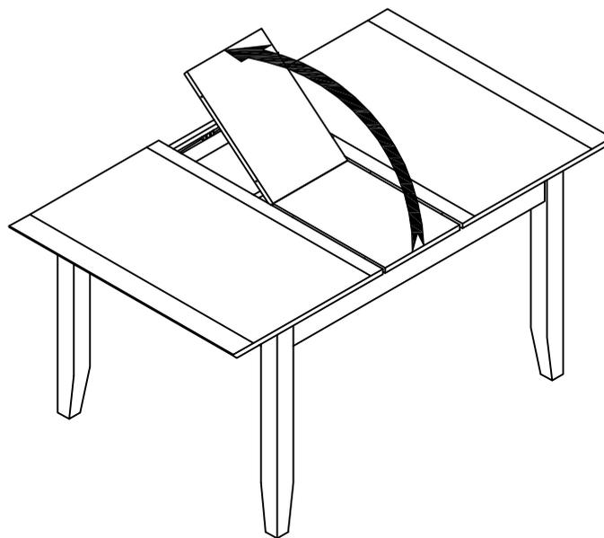
**Step 6** : -Close the top table by sliding both sides of the main table top toward the leaf as shown. Ensure the metal pins are aligned to the holes on the main table top and the leaf before closing the table.
