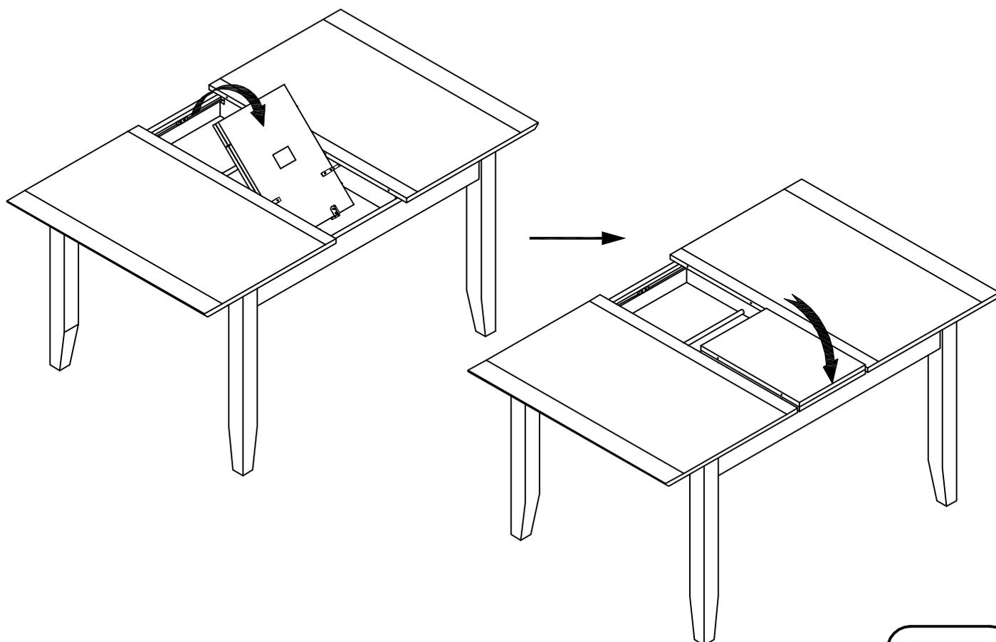
**Step 5** : Extend the leaf by turning the top layer of the leaf all the way open as shown.
