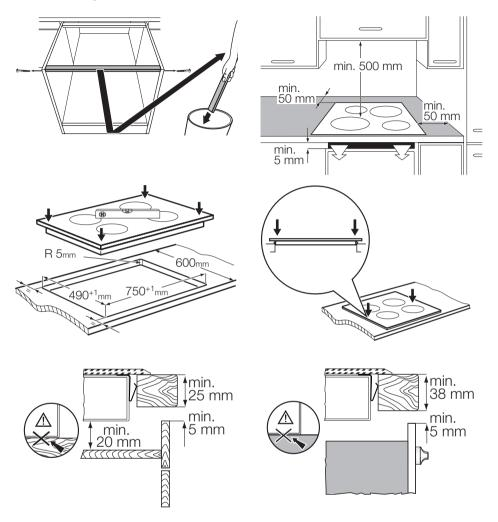
If you use a protection box (additional accessory), the front ventilation space of 5 mm and protective floor directly below the appliance are not necessary.
