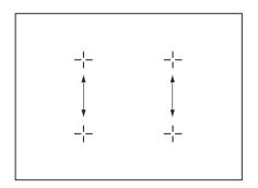
The power management divides the power between two cooking zones in a pair (see the figure). The power function increases the power to the maximum level for one cooking zone in the pair and automatically decreases in the second cooking zone to a lower power
