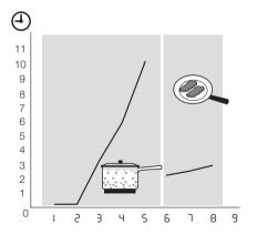
You can get a necessary heat setting in a shorter time if you activate the Automatic Heat Up function. This function sets the
