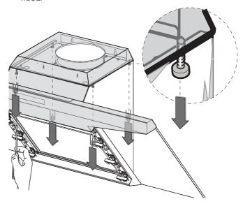
9 Remove the lid and detach the grid from the air outlet hole.
