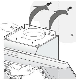
7 Insert the bottom two screws (A) and and tighten.
