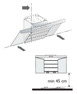
2 Place the fixing template against the wall, lining the bottom holes up with the line drawn in step 1.
