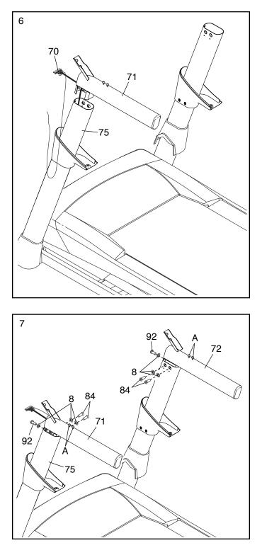
Attach the Left Handrail (71) to the Left Upright (75) with two 5/16" x 1" Screws (84), a 5/16" x 1" Button Head Screw (92), and three 5/16" Star Washers (8). Do not tighten the Screws yet.
