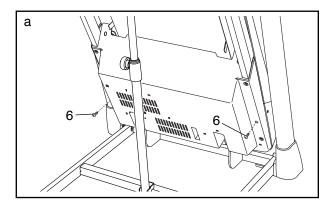
Lower the treadmill (see HOW TO LOWER THE TREADMILL FOR USE on page 27). Remove the three #8 x 3/4" Screws (6). Carefully slide the Motor Hood (57) off.
