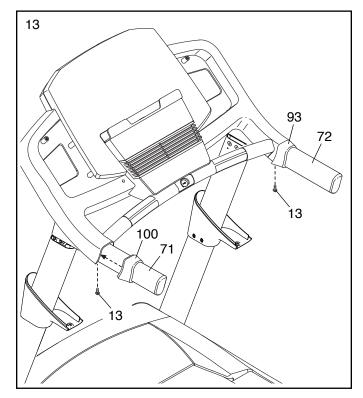
14. Hold the Left Upright Cover (107) against the console assembly. Align the holes in the Left Upright Cover with the holes in the Left Upright (75). Attach the Left Upright Cover with three #8 x 1/2" Screws (13) as shown.
