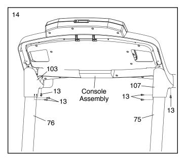
Attach the Left and Right Trays (97, 85) to the console assembly with four #8 x 1/2" Screws (13).
