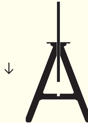
2.1 Turn the circular stool seat upside down, placing the top face down on a hard, smooth surface. Avoid rough surfaces that can scratch the seat. 2.2 Turn the joined two A-shaped legs upside down. Place them on the seat with screw holes of both sections aligned.
