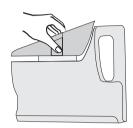
■ After cleaning, dry both parts of the insert thoroughly before replacing it in the water container. When replacing the insert, guide it in at an angle ① and then push it downwards ② as illustrated.
