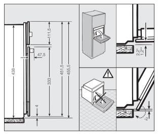
\* Appliances with glass front \*\* Appliances with metal front The appliance must not be operated until it has been correctly installed in its housing unit. Otherwise it poses an electric shock hazard.
