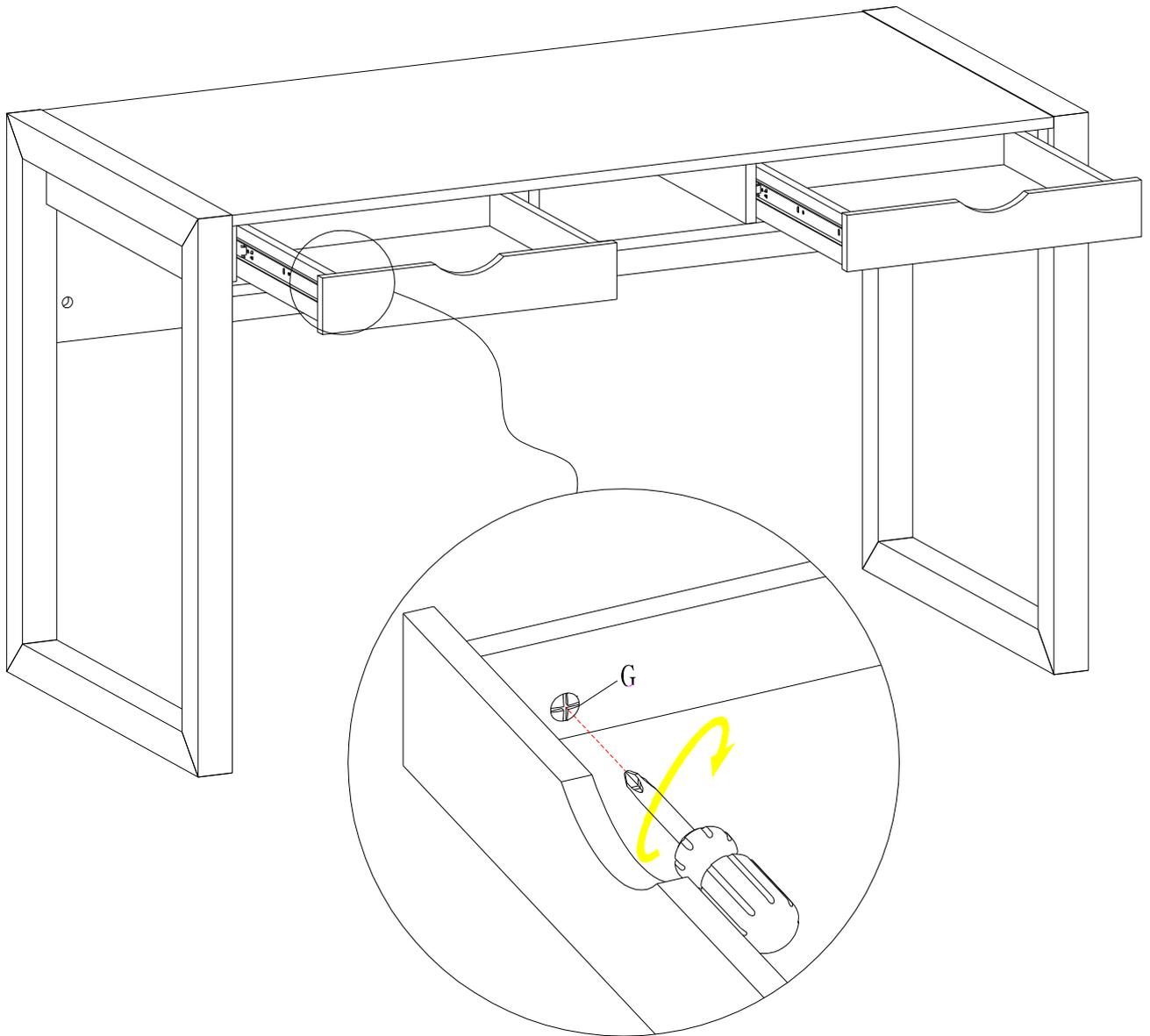
Slide the 2 drawers back into the top section securing the runners with the supplied screw (G).
