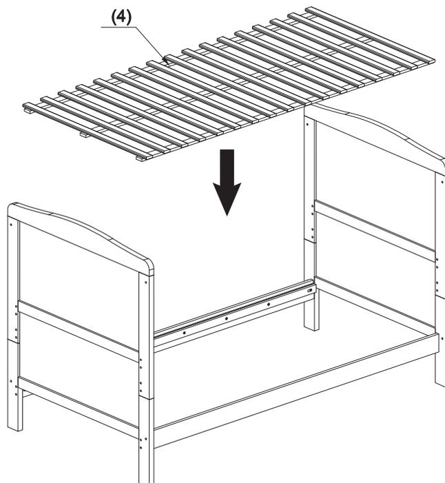
The cot has a choice of three mattress base positions. The lowest base position is the safest, and should be used as soon as your baby is old enough to sit up.
