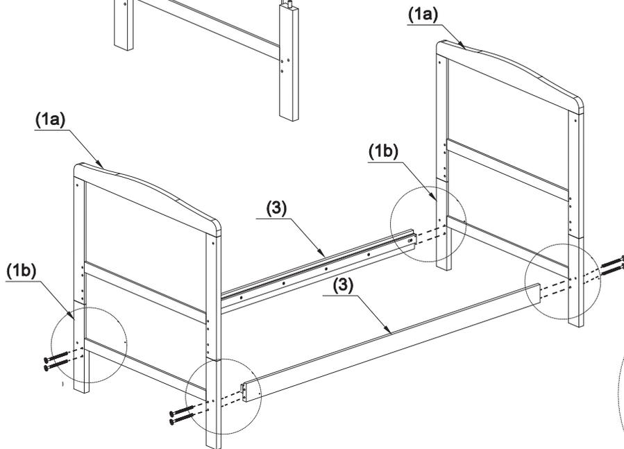
Use the hex key provided (C) to engage the bolt (A) into the barrel nut (B), place the mattress base (part 4) onto the frame and tighten the bolts (A) to secure the mattress base into position.
