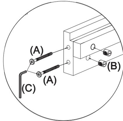
Use the hex key provided (C) to engage the bolt (A) into the barrel nut (B), place the mattress base (part 4) onto the frame and tighten the bolts (A) to secure the mattress base into position.
