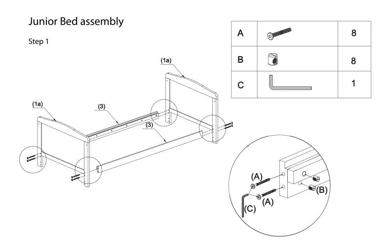
Use the hex key provided (C) to engage the bolt (A) into the barrel nut (B), place the mattress base (part 4) onto the frame and tighten the bolts (A) to secure the mattress base into position.
