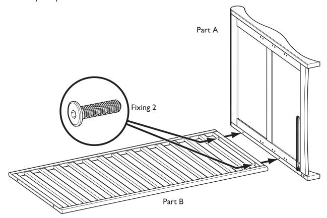
Take one End panel (Part A) and lay it on edge as shown on a soft surface with the drawer runner nearest the floor.
