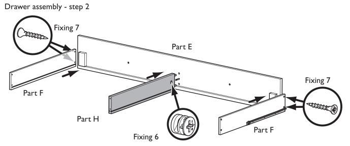
Push the Drawer centre (Part H) onto the Cam pin (Fixing 5) that was fitted to the Drawer front (Part E) in the previous stage. Ensure that the slots in both parts line up with each other.
