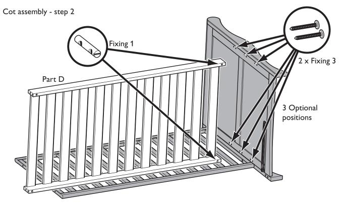
Push two barrel nuts (Fixing 1) into the holes in the underside edges of the base (Part D) so that the slot in the end is visible and is in line with the base rail. If it is not, use a flat-bladed screwdriver to correct it.
