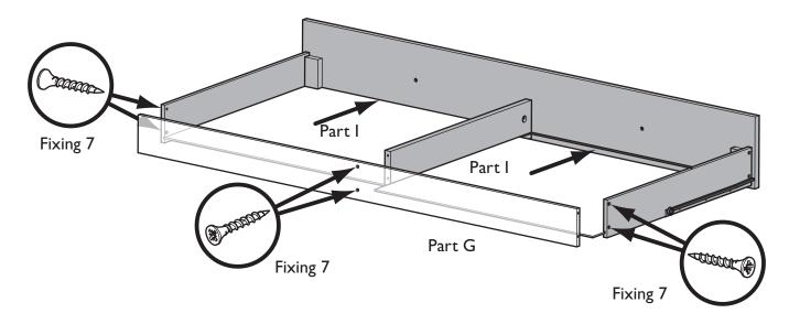
Slide the two Drawer bases (Parts I) into the slots in the assembled drawer.
