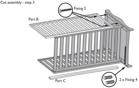
Attach the second Side panel (Part B) using two 45mm bolts (Fixing 2). Do not fully tighten bolts. Push two Dowels (Fixing 4) into the holes in the lower leg of the End panel (Part A) and then attach the Drawer trim (Part C) by pushing it onto the Dowels. Ensure that the curve in this part is on the lower edge.
