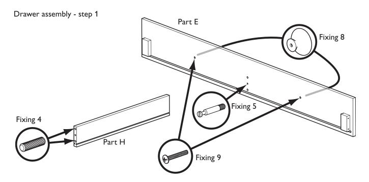
Push two dowels (Fixing 4) into the holes in the end of the Drawer centre (Part H). Attach the Drawer handles (Fixing 8) to the Drawer front (Part E) with the two Handle screws (Fixing 9). Screw the Cam pin (Fixing 5) into the centre hole in the Drawer front (Part E).
