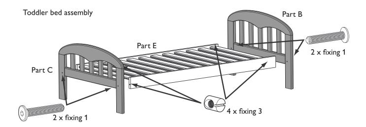
To assemble as a toddler bed, insert four 13mm barrel nuts (fixing 3) into the holes at each corner of the base (part E). Make sure that the slots are visible and, if necessary, use a flat-headed screwdriver to ensure that the slots point towards the holes in the ends. Attach the headboard (part B) and footboard (part C) using four 65mm bolts (fixing 1).
