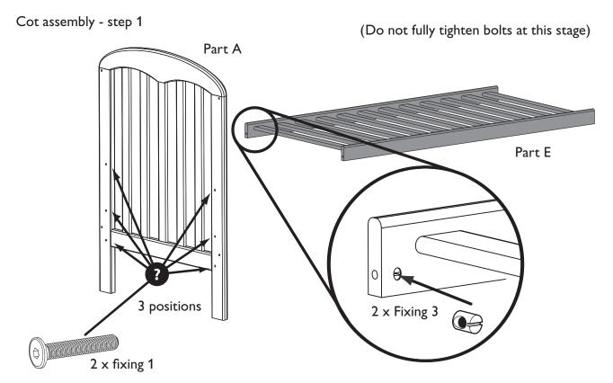
Push two 13mm barrel nuts (fixing 3) into the holes in the base (part E) as shown above. Make sure that the slots are visible and, if necessary, use a flat-headed screwdriver to ensure that the slots point towards the holes in the ends as shown. Select one of the 3 base heights and attach the cot end using two 65mm bolts (fixing 1).
