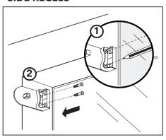
**B.** Using a tape measure and level, whilst using the wall bracket as a guide, mark the position of the brackets on the wall as shown.
