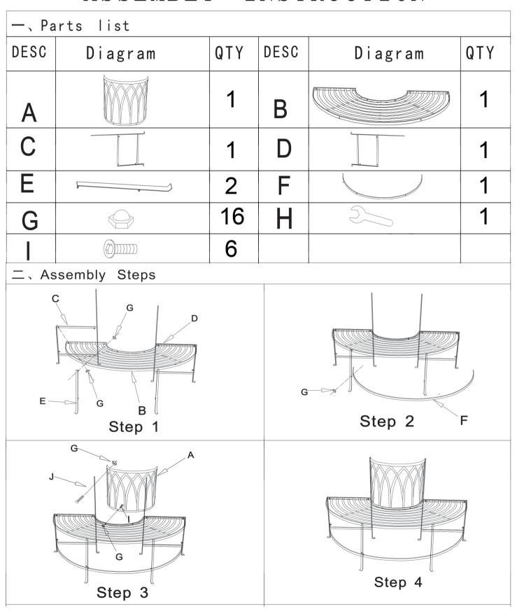
NOTE: Find the screw caps already attached to the bolt section. Please remove these first then assemble the product as per Instruction.
