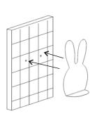
Place hook in desired location and ensure it is level Mark mounting hole locations Drill holes and insert rawl plugs Insert screws into rawl plugs leaving 5mm overhang
