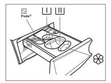
C - Compartment for detergent pods (Max 2 pods). When using detergent tablets, make sure that the Pods® option is activated.
