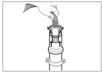
Without the plastic hose guide, to a sink spigot - Put the drain hose in the spigot and tighten it with a clamp. Refer to the illustration.
