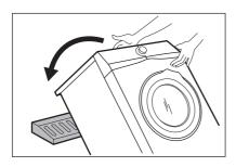
7. Remove the polystyrene protection from the bottom.
