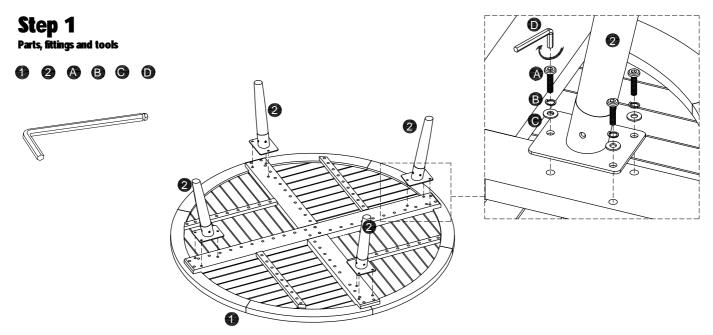
Find a clear area for assembly, near where you intend to use the table. Place table top (1) upside down on a soft surface. Then locate the legs (2) and secure using the Allen bolt (A), Lock washer (B), Washer (C) tightening with the Allen key (D) provided. Repeat this process for all legs.
