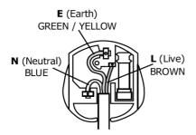
be connected to the terminal marked L (Live), or coloured Red.
