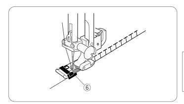
This stitch is ideal for finishing edges of stretch fabrics. It seams and finishes the fabric edges simultaneously. Place the edge of the fabric next to the guide of foot and sew while guiding the fabric edge along the guide.
