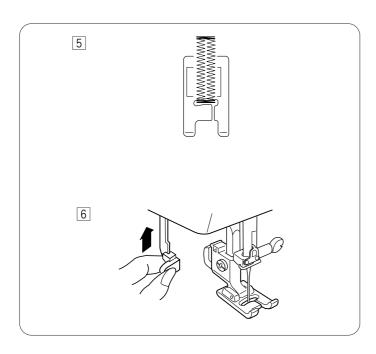
5 Restart the machine to sew the back bartack and right row, and then stop the machine at the starting point.
