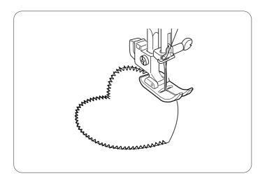
Baste appliqué pieces on the fabric, or fuse the appliqué pieces with an iron-on fabric joiner.
