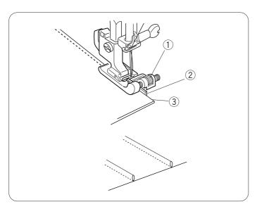
Fold a fabric wrong side together and Lower the needle into the fabric 0.1 - 0.2 cm inside the folded edge.
