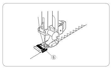
Overcasting is used to prevent fabrics from raveling at raw edges. It can be used to finish a hem edge. Place the edge of the fabric next to the guide of foot and sew while guiding the fabric edge along the guide.
