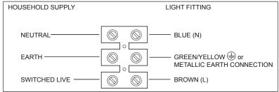
Ensure wiring connections are tight. Ensure earth wire is correctly fitted to the earth connection. Make sure the incoming mains cable is kept away from the heat of the lamp and that the grommet is still in place to maintain the IP rating.
