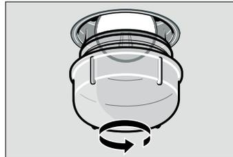
3. Replace the oven light bulb with a bulb of the same type.
