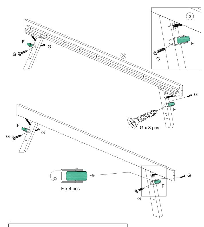
CAUTION: Please do not place the truckle upon its side as it features a spring mechanism that could cause injury.
