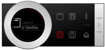
6. Press the start/stop button ▷ to start. The cooking time counts down on the display.
