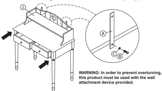
**PLEASE NOTE:** Wall fixings are not supplied with this product as different wall materials require different types of fixing devices. You must use fixing devices that are suitable for the type of wall you intend to mount this product to. The screw supplied is to fix the strap to the dressing table.
