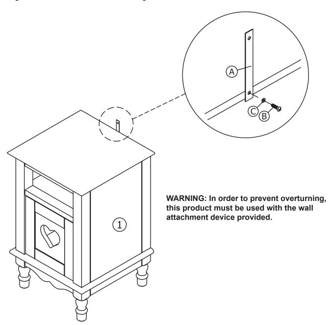
**PLEASE NOTE:** Wall fixings are not supplied with this product as different wall materials require different types of fixing devices. You must use fixing devices that are suitable for the type of wall you intend to mount this product to. The screw supplied is to fix the strap to the bedside.
